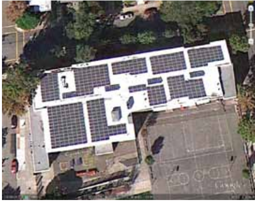
Washington Elementary in Berkeley, CA after installation of a 103 kW rooftop system.
